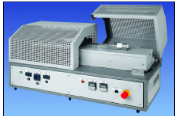
THERMAL CYCLING TEST FURNACE TO CYCLE THERMOCOUPLES BETWEEN UP TO 1200°C & AMBIENT FOR 1000S OF CYCLES
